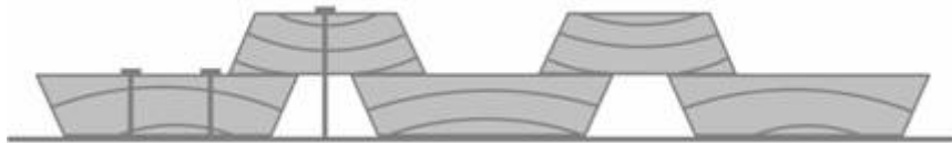
Figure 1 (Board & Batten in cross section)
